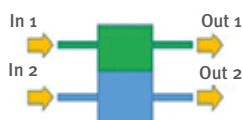
Tangential flows configuration: 2 parallel flows for tangential stimulation of the cells seeded onto the membrane
